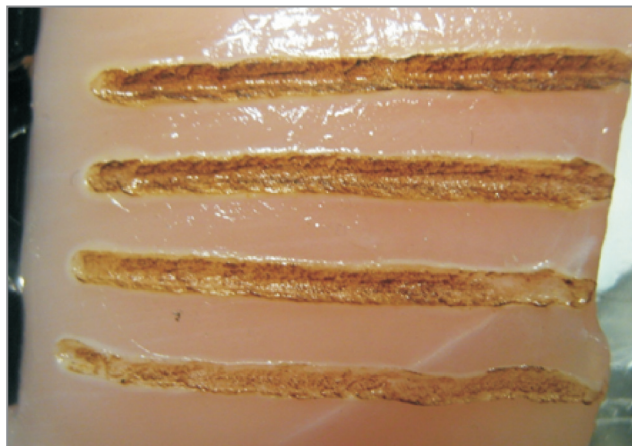
Fig. 3. Linear incision made by the exposure of the chicken muscular tissue to 810 nm laser radiation; power (downward): 9, 7, 5, 3 W (macrophotograph)
