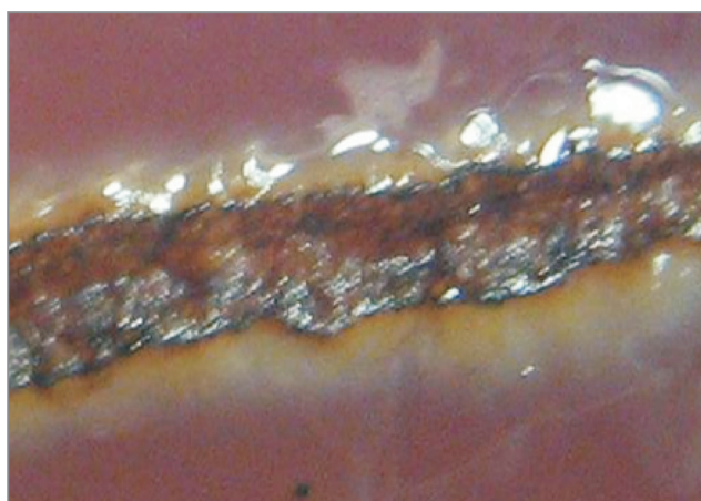
Fig. 4. Assessment of ablation zone and lateral coagulation zone on the cattle liver tissue (macrophotograph)
